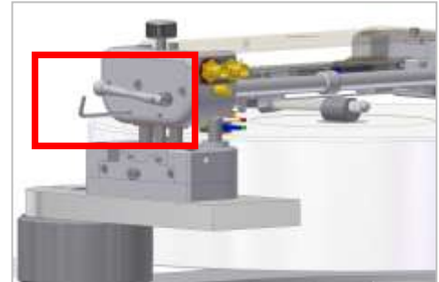
Pic.15: Adjustment of the tonearm
